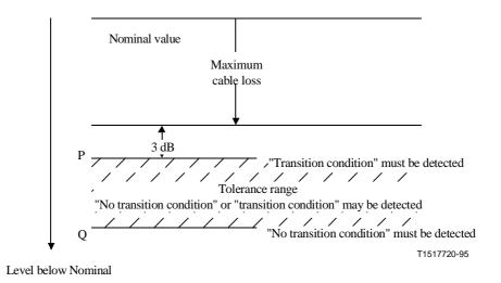
NOTE 1 – The signal level P is (maximum cable loss +3) dB below nominal.
